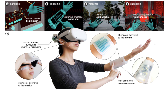
Figure 1: We propose a novel haptics approach, which we call Chemical Haptics , based on delivering topical stimulants to the user's skin. Upon absorbing these stimulants, receptors in the user's skin are chemically triggered, rendering distinct haptic sensations. To explore our approach in interactive contexts, such as VR, we engineered a self-contained wearable that delivers liquid stimulants. Here, it allows this VR user to feel four haptic sensations: (a) Sanshool creates tingling, which renders electric sparks emitted from a "short-circuiting" touchscreen on the arm; (b) Lidocaine creates numbing, which renders a malfunctioning arm interface by reducing tactile feedback as the user taps the buttons; (c) Menthol creates cooling, which renders cold winter air on the face; finally, (d) Capsaicin creates warming, which renders the hot air on the face from a nuclear reactor on the brink of meltdown.
