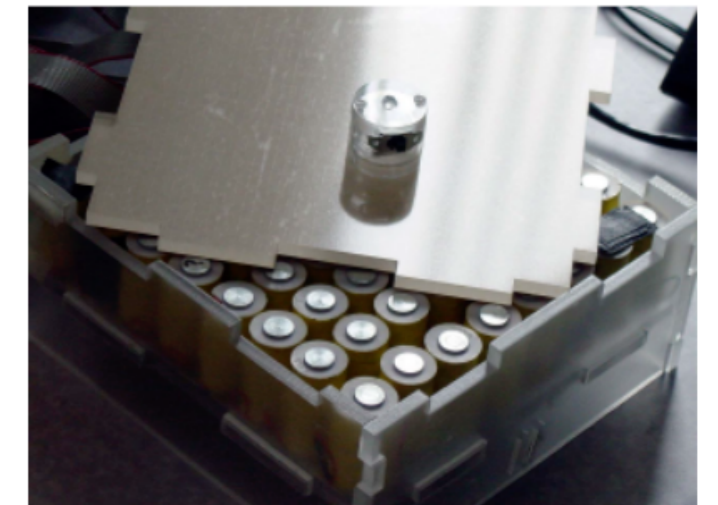
Figure 1. The Actuated Workbench uses a grid of electromagnets to move a magnetic puck across a table surface.
