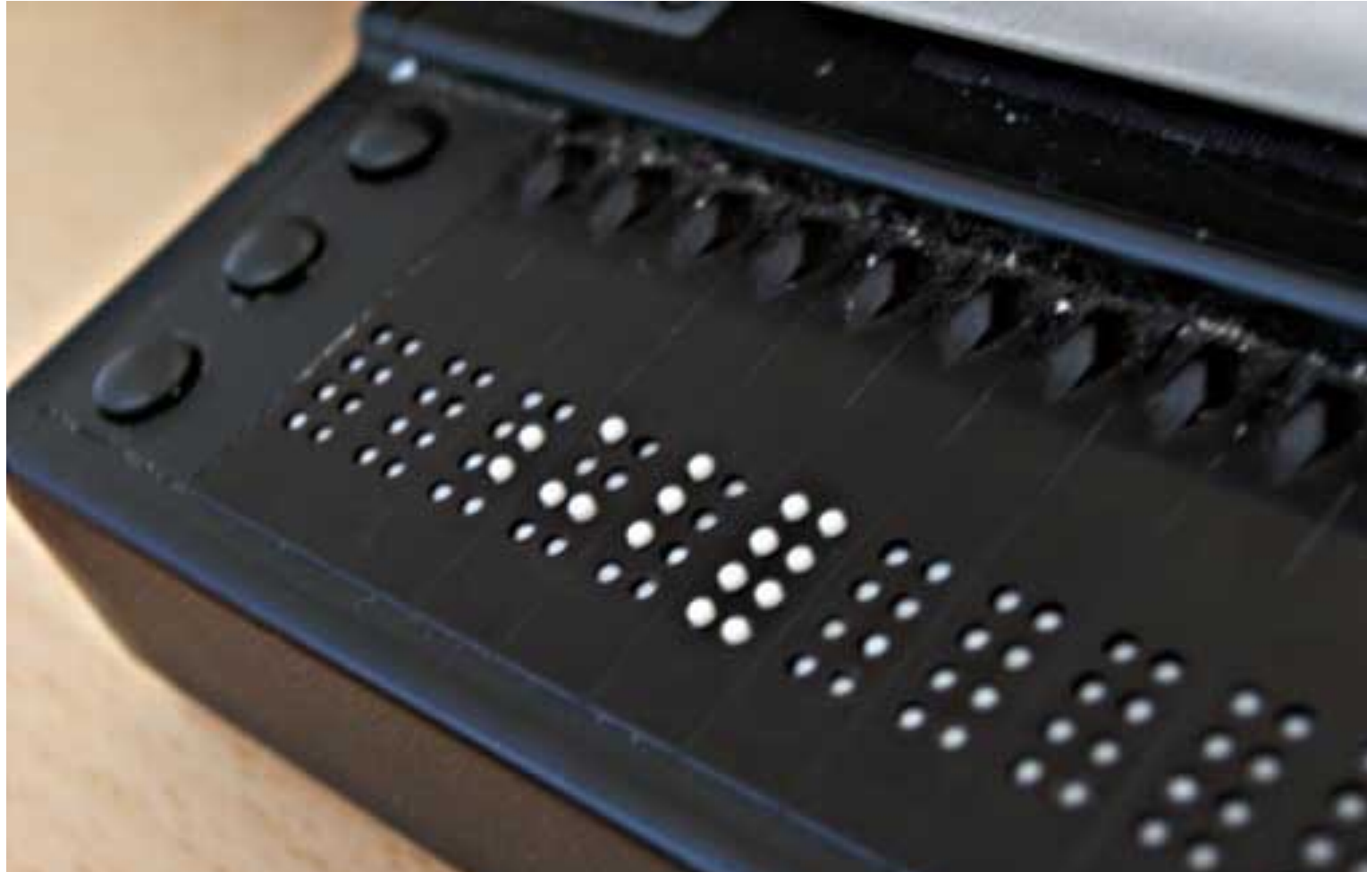
1969 braille display for the blind and visually impaired
