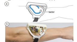
Figure 1: Skin drag displays drag a tactor over the wearer's skin in order to communicate a spatial message, (a) e.g. write a "C" on the user's arm. (b) Our self-contained prototype.
