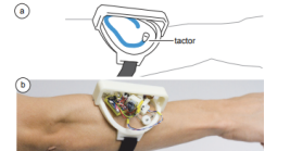
Figure 1: Skin drag displays drag a factor over the wearer's skin in order to communicate a spatial message. (a) e.g. write a "C" on the user's arm. (b) Our self-contained prototype.
