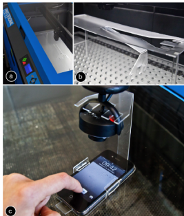
Figure 1: LaserOrigami fabricates 3D structure by bending, rather than using joints, thereby eliminating the need for manual assembly. Here it fabricates a mobile phone screen cam by (a) cutting the contour lines and (b) heating up the bend paths until the material
