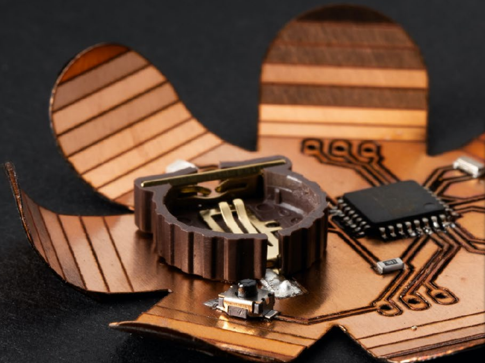
Figure 1: Fibercuit overview. a) Our fiber laser engraver setup with a custom rotary table. b) Cutting the conductive layer on our custom composite using the fiber laser. c) A kirigami flower circuit that can function as an Arduino. d) A custom stretchable flex cable. e) A kirigami crane with a battery holder and 2 LEDs.
