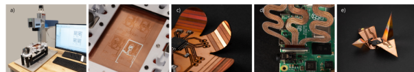
Figure 1: Fibercuit overview. a) Our fiber laser engraver setup with a custom rotary table. b) Cutting the conductive layer on our custom composite using the fiber laser. c) A kirigami flower circuit that can function as an Arduino. d) A custom stretchable flex cable. e) A kirigami crane with a battery holder and 2 LEDs.
