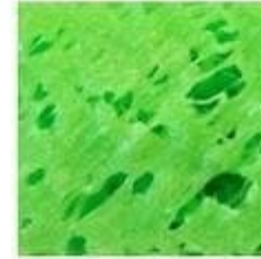
HOLES OR GAPS IN TOP LAYER
