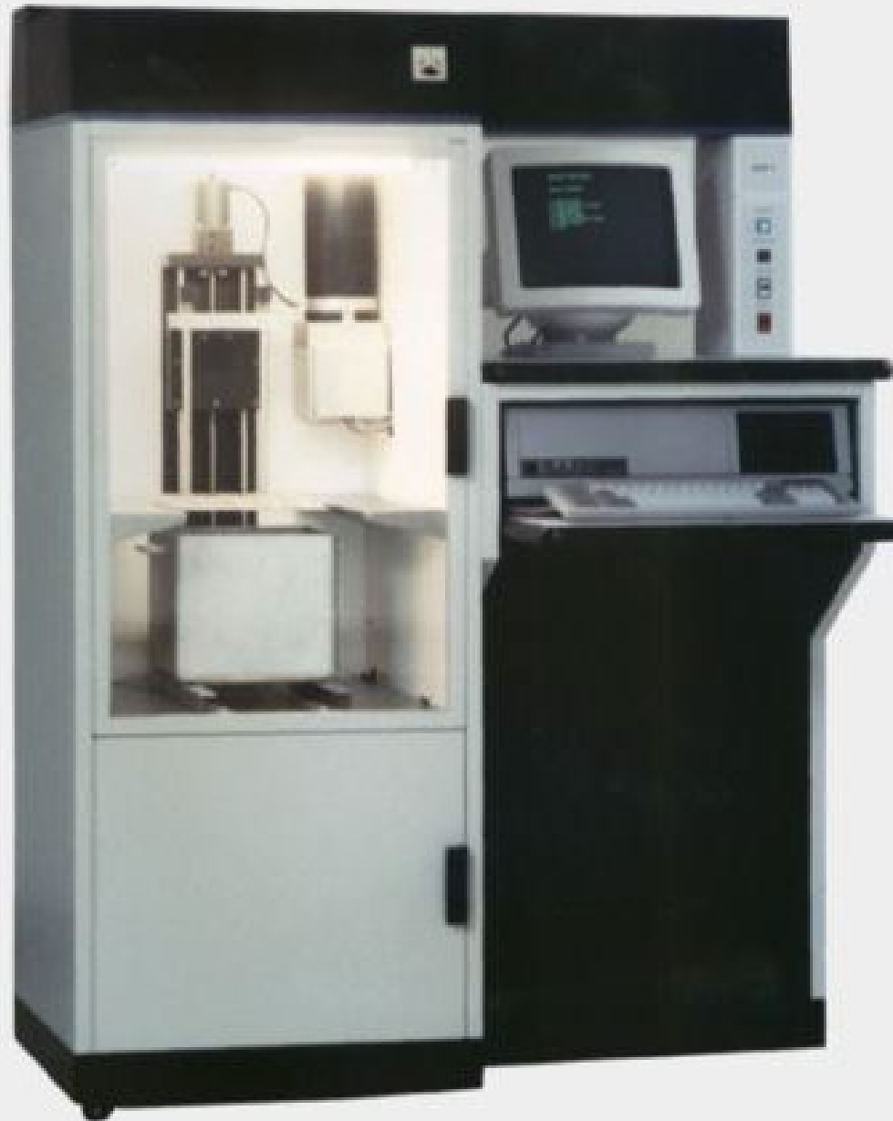
The first commercial 3D printer SLA-1 printer 1987
