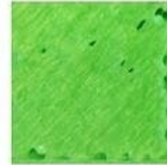
GAPS BETWEEN INFILL AND OUTLINE
