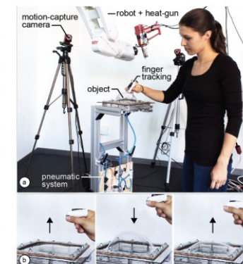
Figure 1: (a) FormFab changes the workpiece continuously while the user is interacting with it. First, a heat-gun warms up the workpiece. Once the material has become compliant, (b) the user's hand gesture interactively controls a pneumatic system that applies pressure or vacuum, pushing the material outwards or pulling it inwards.
