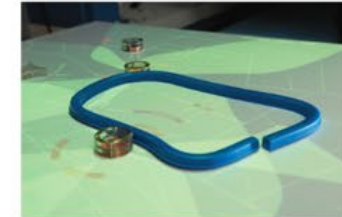
Figure 1: A flexible “artist’s curve” constraining the motion of a cellphone tower in the Pico system.
