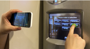
Figure 1. StateLens is a system that enables blind users to interact with touchscreen devices in the real world by (i) reverse engineering a structured model of the underlying interface, and (ii) using the model to provide interactive conversational and audio guidance to the user about how to use it. A set of 3D-printed accessories enable capacitive touchscreens to be used non-visually by preventing accidental touches on the interface.
