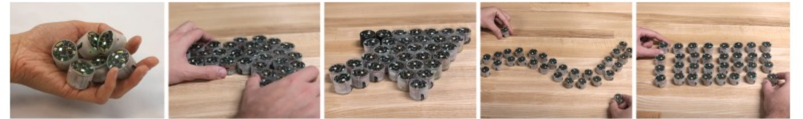
Figure 1. Zooids can be held as tokens, manipulated collectively or individually, behave as physical pixels, act as handles and controllers, and can move dynamically under machine control. They are building blocks for a new class of user interface we call swarm user interfaces .
