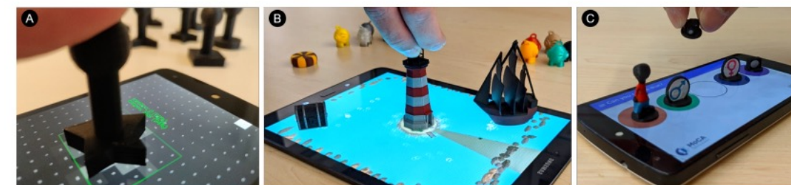
Figure 1: Itsy-Bits recognizes 3D-printed tangibles as small as a fingertip via the capacitive image of an embedded conductive shape (A). This opens up a variety of tangible user interfaces on the most common form factors of touchscreens, such as individualized interactive board games (B) or a more tangible learning experience (C).
