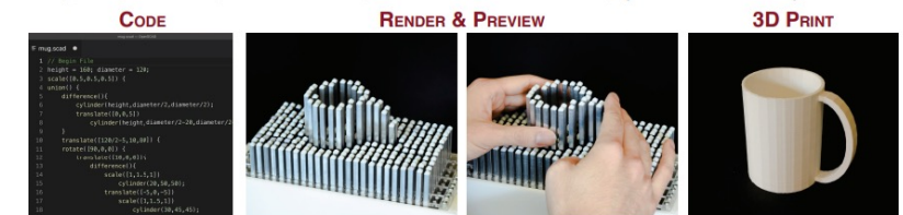
Figure 1. We investigate an accessible 3D modelling workflow (shapeCAD) where 3D models are generated through OpenSCAD, a declarative programming language for 3D modeling, and rendered at interactive speeds in a 2.5D shape display consisting of a grid of 12 \times 24 actuated pins.
