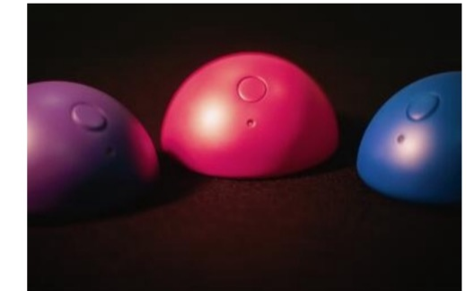
Figure 1: Three palm-sized curlybots (each with a large record/playback button and a small indicator light).
