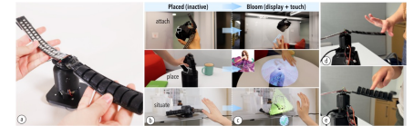
Figure 1: (a) BloomBeacon is a mobile, expansive touch display based on Persistence-of-Vision motion that ‘blooms’ from soft, line-like blades. When inactive, it is relatively compact, allowing it to be (b) easily placed in the environment. (c) When Blooming, a touch surface emerges from the line. (d-e) A series of studies was conducted to investigate the key factors that affect touch-sensing performance and user experience.
