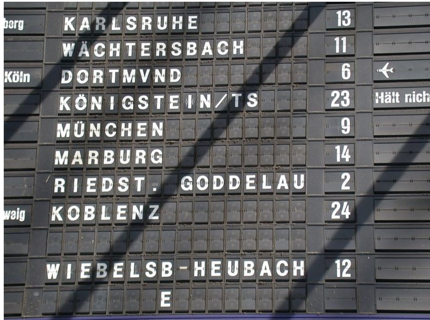
1957 split flap display (electro-mechanical)
