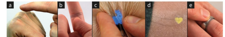
Figure 1: SkinMarks are conformal on-skin sensors and displays. They enable interaction on five types of body landmarks: (a) skeletal landmarks, (b) skin microstructures, (c) elastic skin landmarks, (d) visual skin landmarks, and (e) accessories.
