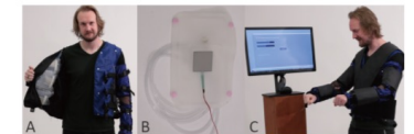
Figure 1. Force Jacket - A: Appearance of Force Jacket; B: Individual airbag with force sensitive resistor; C: User study set-up.
