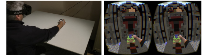
Figure 1. User building a virtual castle by arranging and stacking multiple virtual cubes mapped to a single physical cube.
