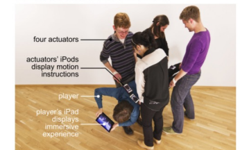
Figure 1: Haptic turk allows producing motion experiences anywhere anytime. Here, the suspended player is enjoying an immersive hang gliding game. The four actuators create just the right physical motion to fill in the player's experience.
