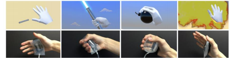
Figure 1. PuPoP is a wearable pneumatic shape-proxy interface for VR capable of popping up to primitive shapes and flattening on the palm. We demonstrate grasping emulation of picking up a virtual Lightsaber with a cylindrical PuPoP and throwing a virtual bomb with a spherical PuPoP.
