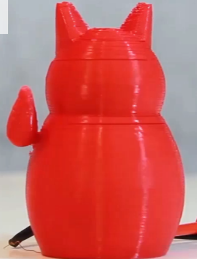
Figure 1. 3D printed electromagnetic devices. a) Solenoid used to actuate the cat hand; b) A Ferrofluid display; c) A movement sensor based on coupling strength; d) The stator and the rotor of a reluctance motor. The electromagnetic components are printed with a soft iron core, wound in place, and multiple layer of copper wire.
