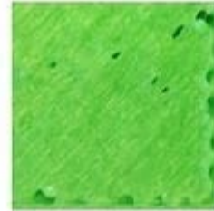
GAPS BETWEEN INFILL AND OUTLINE
