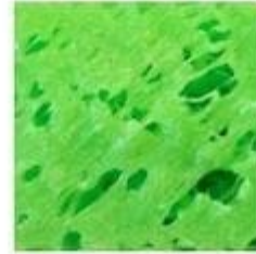
HOLES OR GAPS IN TOP LAYER
