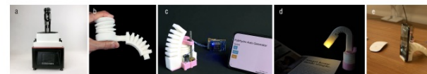
Figure 1: FabHydro overview: a) an off-the-shelf SLA printer with a modified tank and printing plate; b) a complete hydraulic device with a bellows generator and a bending actuator connected with a short piece of tubing; c) a bending actuator is activated by an automatic generator; d) a printed lamp lights up with the change of its posture; e) a phone stand acts as an ambient display when the phone rings.
