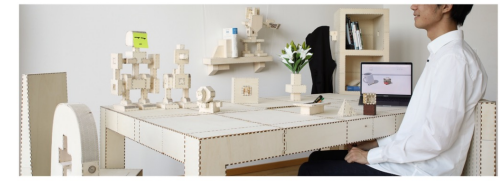
Figure 1: A selection of objects created using kyub, a software system that allows users to design 3D objects for laser cutting. By affording closed box structures, objects made using kyub are very strong. This allows users to make tables, shelves, and chairs that can hold a person. (All shown objects are assembled from 1mm plywood sheets—pressure fit, not glued).
