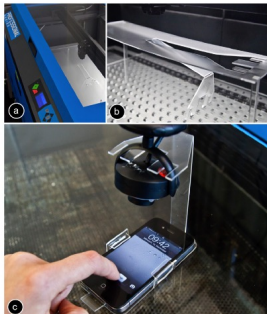
Figure 1: LaserOrigami fabricates 3D structure by bending, rather than using joints, thereby eliminating the need for manual assembly. Here it fabricates a mobile phone screen cam by (a) cutting the contour lines and (b) heating up the bend paths until the material becomes compliant and bend down under the force of gravity.
