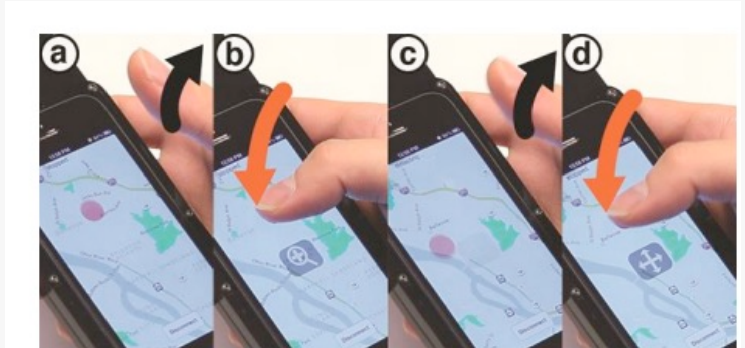
Figure 7. In our map app, raising the finger ‘high-up’ (a, c) before touch down switches between pan/zoom modes (b, d).
