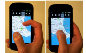
Figure 1. (left) It is difficult for a user to perform interactions like pinch-to-zoom with one hand. (right) GripSense senses user's hand posture and infers pressure exerted on the screen to facilitate new interactions like zoom-in and zoom-out.
