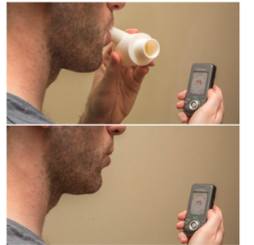
Figure 1. A user using SpiroCall on a feature phone (Sony w580) with, and without a SpiroCall whistle.
