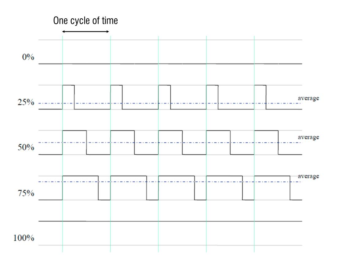
analogWrite() is on a scale of 0 (always off) – 255 (always on) Pins that support PWM: all GPIO pins except 6-11 and 34-39
