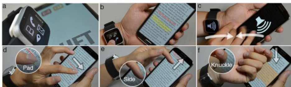
Figure 1. A duet of interaction between a handheld and a wrist worn device (a): the watch is used as a tool palette when annotating text on the phone (b); a simultaneous pinch-to-close swipe gesture on both devices mutes their notifications (c); the watch's orientation indicates which hand part causes a touch, thus enabling a seamless transition between modes: for example, writing with the pad of the finger (d), scrolling with side of the finger (e), and text selection with the knuckle (f).
