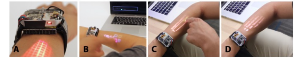
Figure 1. Our self-contained projection smartwatch (A) provides rectified graphics with touch input on the skin (B). We use a slide-to-unlock mechanism to reject inadvertent touches and provide a rapid projection calibration (C) before apps can be used (D).
