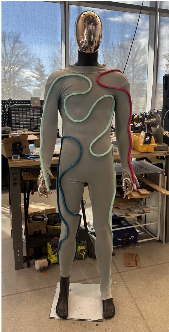
Figure 3: The performer’s costume on a mannequin. Three pieces of silicone track is sewn onto the dancer’s leotard. The dancer can move the robot between different pieces of track.
