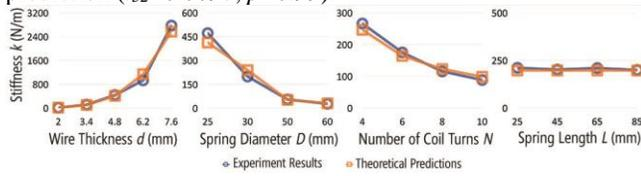
Figure 6. Experiment 2 results showing that 3D-printed helical springs perform similarly to theoretical predictions as measured by a load frame with different  $d, D, N$ , and  $L$  values.
