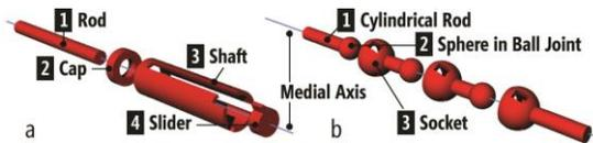
Figure 16. An exploded view of (a) a prismatic joint and (b) a chain of ball joints, which are used for *linear-only* and *twist+bend* respectively.
