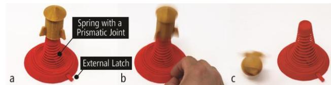
Figure 18. A launching rocket application: (a) a rocket sits on top of a compressed "smoke" spring, which is locked by an external latch; (b) the user can launch the rocket by pulling the latch; and (c) the smoke is in its full extension.
