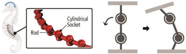
Figure 10. A chain of knuckle joints used for *bend-only* deformations.
