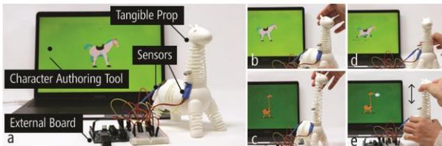
Figure 20. The setup of a tangible storytelling prop.
