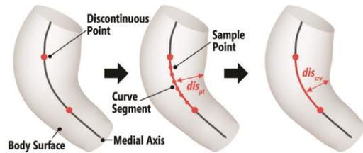
Figure 13. Generating the medial axis, calculating the size of the selected body, and evaluating the printability of an embedded spring.
