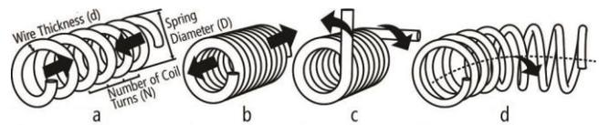
**Figure 2. Basic helical spring deformation behaviors: (a) compress, (b) extend, (c) twist, and (d) laterally bend.**
