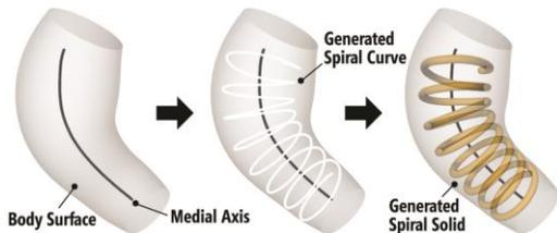
Figure 14. Generating the deformation spring using the generated medial axis and *RhinoCommon* functions.
