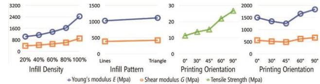
Figure 5. Experiment 1 results showing that  $E$  and  $G$  increase with infill density as well as more robust infill patterns. Tensile strength increases as printing angle increases; however, shear stress is highest at 45°.
