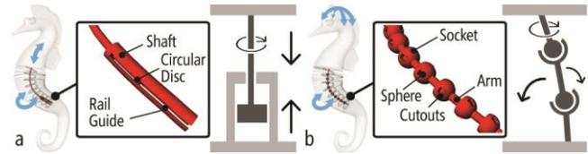
Figure 11. (a) A cylindrical joint is used for *linear+twist* deformations and (b) a chain of ball joints is used for *twist+bend* deformations.
