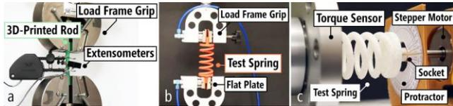
Figure 3. Mechanical experiment setups: (a) the load frame stretches a 3D-printed rod; (b) the load frame stretches a 3D-printed helical; and (c) the motor rotates a helical spring and torque is measured.
