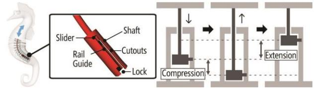
Figure 8. A prismatic joint is used for a *linear-only* deformation.
