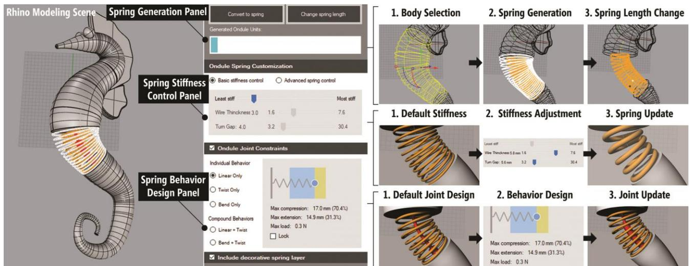
Figure 12. The *Ondulé* spring design tool interface (left) has four parts: Rhino modeling environment, a spring generation panel, a spring stiffness control panel, and a spring behavior design panel. The workflow for each design panel is shown on the right.
