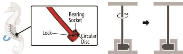
Figure 9. A revolute joint is used for a *twist-only* deformation.
