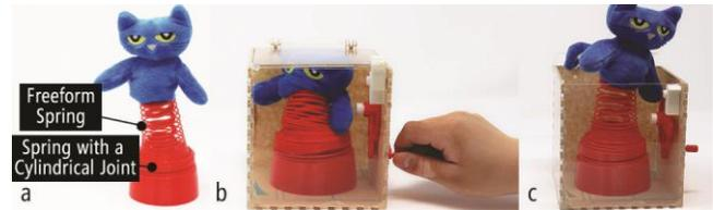
Figure 17. A jack-in-the-box spring mechanism generated by *Ondulé*: (a) two spring designs are embedded; (b) the cat can be fully compressed and locked inside a laser-cut box; and (c) the cat pops out following a path as a surprise.
