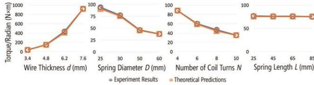
Figure 7. Experiment 3 results showing that 3D-printed helical springs have similar twisting performance to theoretical predictions with varied  $d, D, N$ , and  $L$  values.
